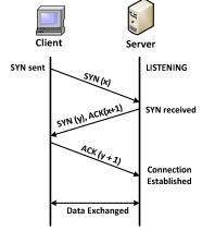
Fig. 2 TCP 3-way handshake
