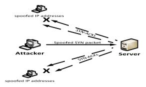
Fig. 5 Spoofing-based attacks
