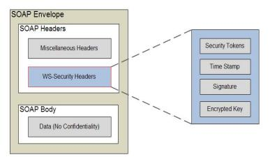
Figure 1. WS-Security for SOAP Message (Authentication and Integrity)
