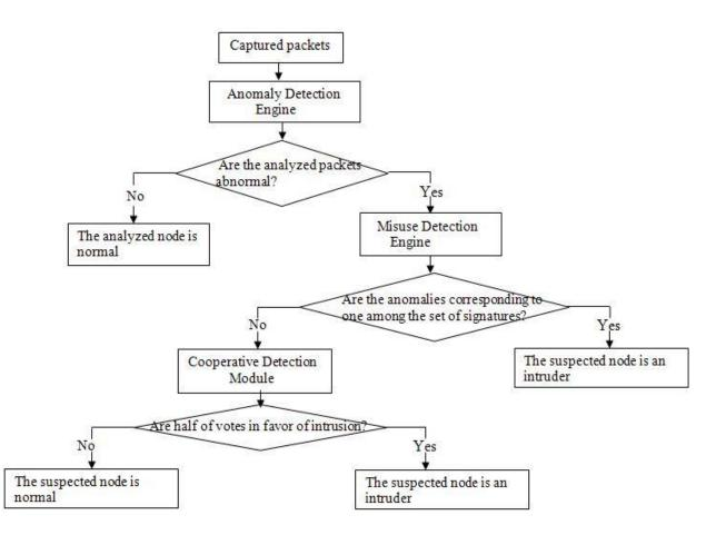
Figure 4. The flowchart of IDS framework in WSN
