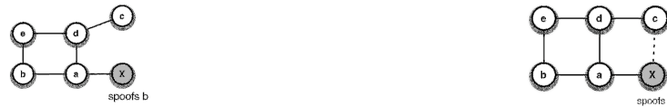
(a) The gray malicious router spoofs b (b) X spoofs b and advertises a link to c
