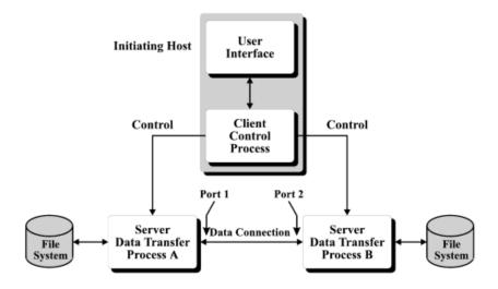
Figure 10. FTP Client Server Process
