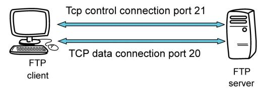
Figure 7. Control and data connection
