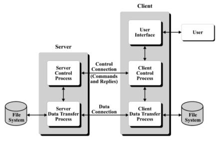
Figure 9. FTP Client-Server Application
