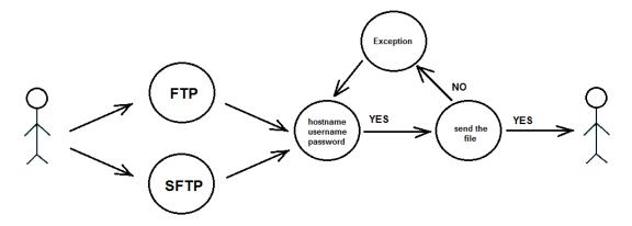
Figure 14. Use case Diagram for Huge Data File Transfer.
