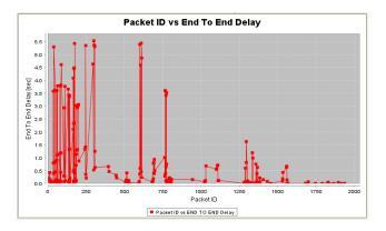
Figure 9: End to End Delay of DSR
