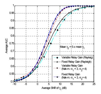
Figure 7. Fixed and variable relay gain performance over fading channels using unified SNR model with u = 2.
