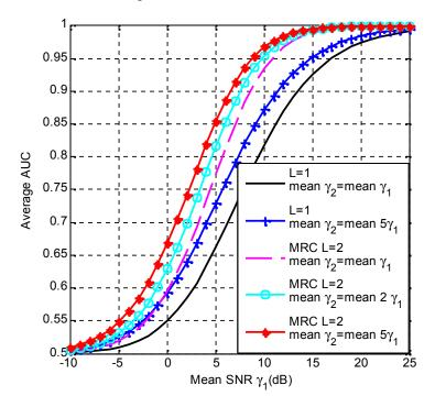
Figure 4. Average AUC vs. mean SNR for two hop fixed gain AF relaying over i.i.d. / i.n.d. Rayleigh fading with MRC illustration (u = 2).
