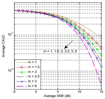
Figure 3. Average AUC vs. mean SNR for a relay network with source to destination direct path over *i.i.d.* Nakagami-m Channels, with m = 2 and u = 3.5.
