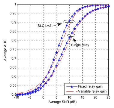
Figure 5. Comparison of fixed and variable relay-gain over i.i.d. Rayleigh channels for a dualhop relay network (u = 2).
