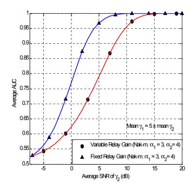
Figure 8. Comparison of variable relay gain and fixed relay gain based spectrum sensing
