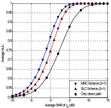
Figure 9. Comparison of MRC (N+1) and SLC (N+1) schemes, fixed gain AF dual-hop relay system over Nakagami-m channels with u = 2.
