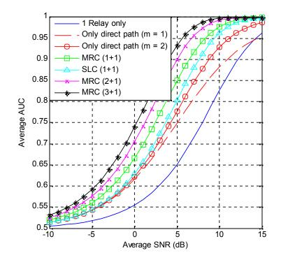
Figure 2. Average AUC vs. mean SNR for N-relay network with source to destination direct path over *i.i.d.* Nakagami-m Channels (m = 2 and u = 3.5).
