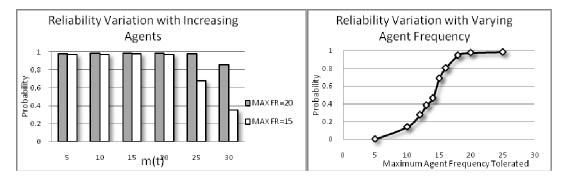
Figure 1. Reliability variation with no.of agents Figure 2. Reliability variation with varying tolerance limit on accepted agent frequency
