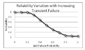
Figure 5.Reliability variation with varying link failure probability
