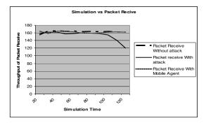
Fig 9 Throughput of Packet receive when the network is under attack and in presence of mobile agent
