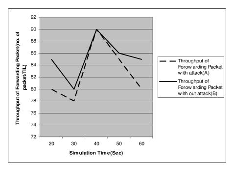
Fig 8 Throughput of forwarding packet when the network is under attack and in presence of mobile agent
