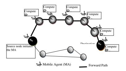
Fig 4: A network Without Malicious Attack The MA moves from source node  $N_0$  to Destination Node  $N_6$  by the forward path.
