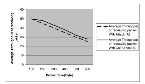
**Fig 6** Average Throughput of Packet receive when the network is under attack and in presence of mobile agent
