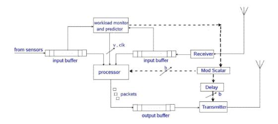
Figure 6. CAP Management Conceptual Block Diagram
