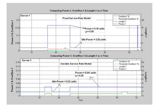
Figure 7. Performance graphs of processor with input buffer with fixed service rate and with variable service rates under normal condition
