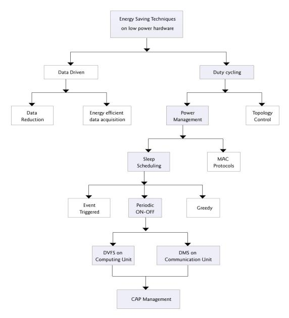
Figure 2. Scope of CAP Management on a Wireless Sensor Node
