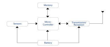
Figure 1. Basic architecture of a sensor node
