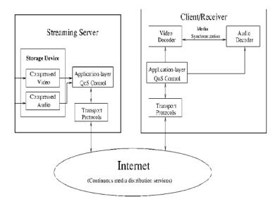
Fig 7 Video transmission module of ENVMT
