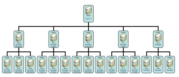
Figure 5. Two hierarchal level for Web Services and Parallel AdaBoost, based on Master and five Sub-Master and 3 Salves for each Sub-Master (Total of twenty one Pc's)
