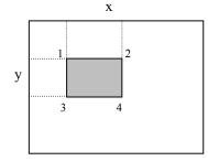
Figure 2. Calculating the integral image in a rectangular region.
