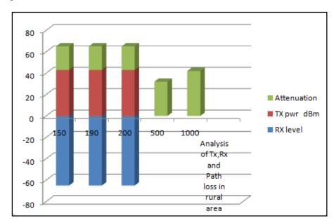
Figure 9.b. Analysis of path loss at rural area
