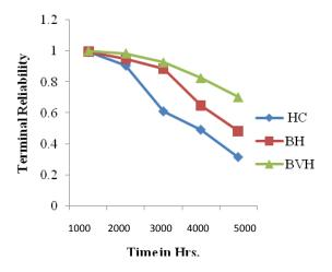
Figure 11: Comparison of Terminal Reliability for p=64
