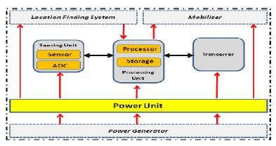
Figure 2. Basic physical architecture of an intelligent sensor
