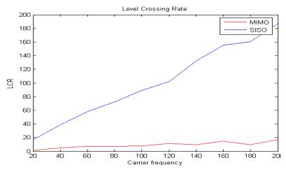
Fig 5a: LCR vs Carrier frequency with differnt channel practically
