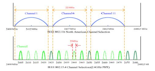
Figure 1. WIFI and Zigbee Overlapping Channels in The 2.4Ghz ISM Band
