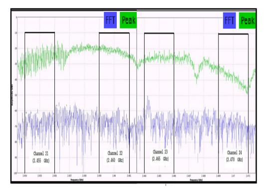
Figure 6. Interference Signal on ZigBee Channels 21, 22, 23, and 24 of Experiment Two
