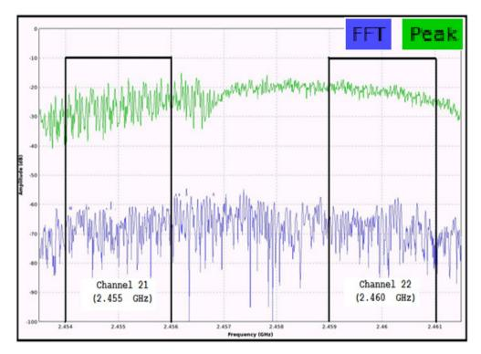
Figure 4. Interference Signal on ZigBee Channels 21 and 22 of Experiment Two
