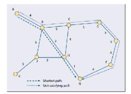
Figure1. A sample QoS Routing in MANET
