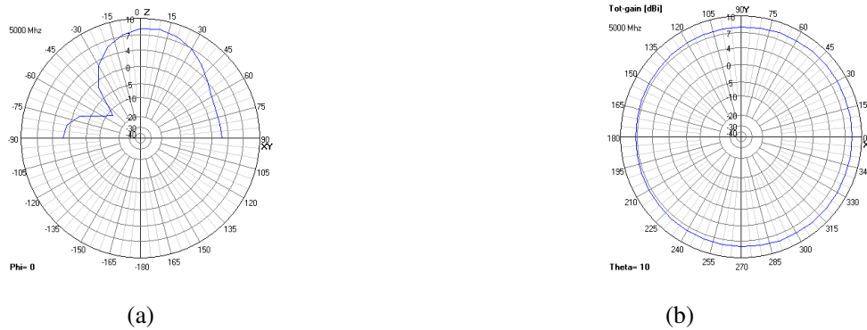
Figure 8. Total Gain pattern of the proposed Inverted-L antenna at 5 GHz in (a) vertical plane (b) horizontal plane
