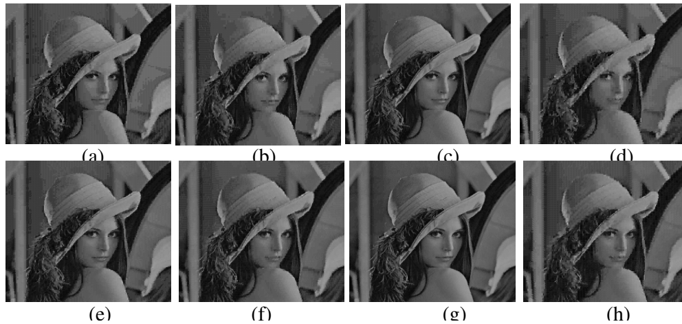
Figure 6: Reconstructed Image from LBG based trained codebook when (a) the codebook size 128 and codeword size 4 \times 8 ; (a) the codebook size 128 and codeword size 8 \times 4 ; (a) the codebook size 256 and codeword size 4 \times 4 ; (a) the codebook size 256 and codeword size 8 \times 8 ; (a) the codebook size 512 and codeword size 4 \times 8 ; (a) the codebook size 512 and codeword size 8 \times 4 ; (a) the codebook size 1024 and codeword size 4 \times 4 ; (a) the codebook size 1024 and codeword size 8 \times 8 ;
