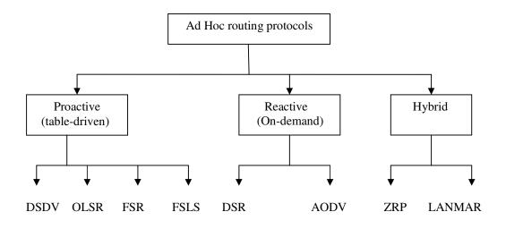
Figure 1. Classification and examples of ad hoc routing protocols.
