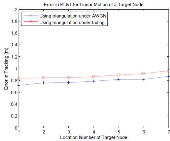
Figure 6: Error of PL&T under AWGN channel and under fading channel for linear motion.
