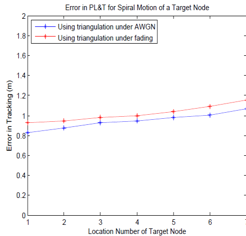
Figure 7: Error of PL&T under AWGN channel and under fading channel for spiral motion.
