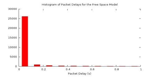
Figure 4. The histogram of the packet delays for the free space loss model
