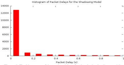
Figure 6. The histogram of the packet delays for the shadowing loss model
