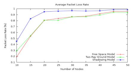
Figure 3. The average packet loss rate for the three propagation models
