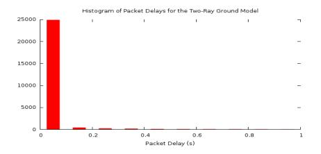
Figure 5. The histogram of the packet delays for the two-ray ground loss model
