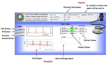
Figure 6. The front panel of the program
