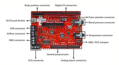
Figure 3. The biometric shield
