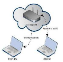
Figure 2. Scenario: Running Snort on client station - system topology
