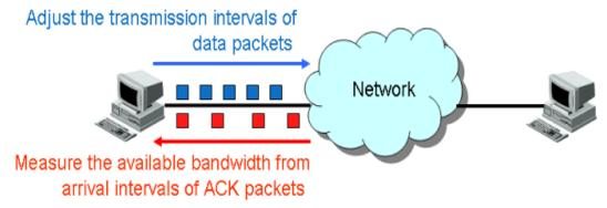
Figure 1. Outline of ImTCP Mechanism
