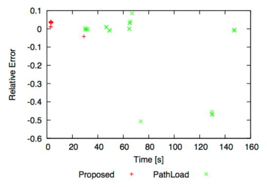
Figure 4. Distribution of the relative errors between measured and actual bandwidth and the measurement time
