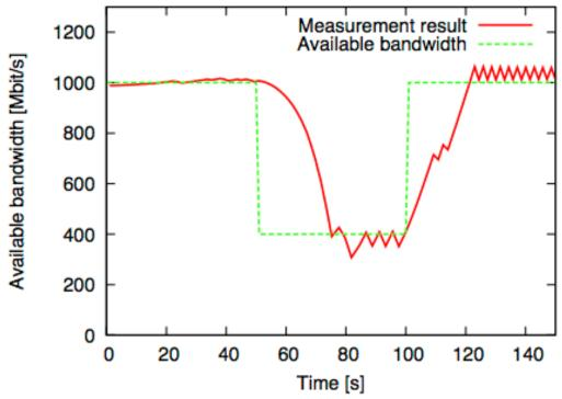
Figure 5. Tracking bandwidth changes in narrow-bandwidth network
