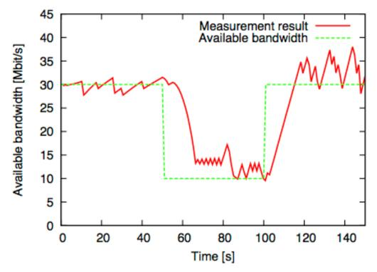
Figure 6. Tracking bandwidth changes in high-speed network
