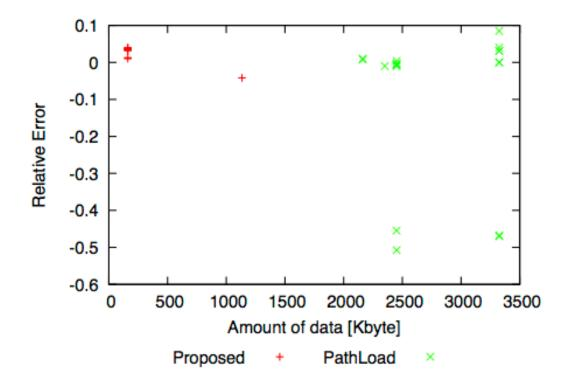
Figure 3. Distribution of the relative errors between measured and actual bandwidth and the total amount of data
