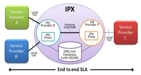
Figure 1. IPX basic network configuration
