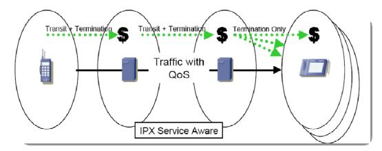
Figure 4. IPX multilateral hub service interconnect model
