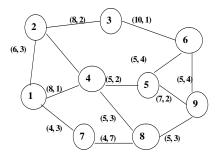
Figure: 5: An Example Network With edges (Bandwidth, Delay)
