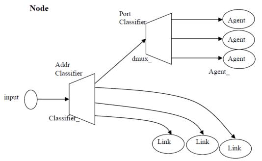
Figure 3: Diagram of a node in NS2.
