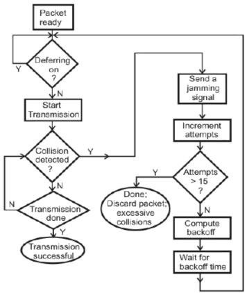
Figure 2: Binary exponential back off algorithm used in CSMA/CD
