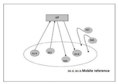
Figure 6: Principle of simulation used to assess the changed Back-off
