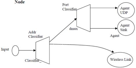
Figure 5: Diagram of the mobile node
