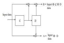
Figure 1. Convolutional Encoder for K=3
