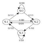
Figure 2. State Diagram of Convolutional Encoder for K=3
