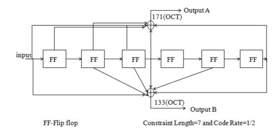
Figure 3. Convolutional Encoder for K=7
